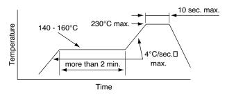
The following soldering patterns are□ recommended for reflow soldering
